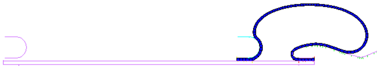
Figure 3.5-6 Deformed Shape of the Axisymmetric Airspring Model
