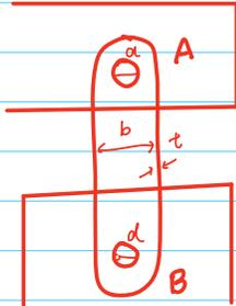
Link AB, of width  $b = 50\text{mm}$  and thickness  $t = 6\text{mm}$ , is used to support the end of a horizontal beam.
