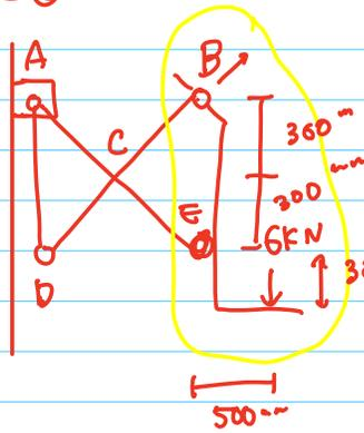
(a) the average shearing stress in the 12-mm-diameter pin at B.
