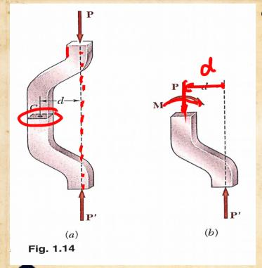
• However, if a two-force member is loaded axially, but *eccentrically* as shown in Fig.1.14a, we find from the conditions of equilibrium of the portion of member shown in Fig.1.14b that the internal forces in a given section must be equivalent to force **P** applied at the centroid of the section and a couple *M* of moment M=Pd.
