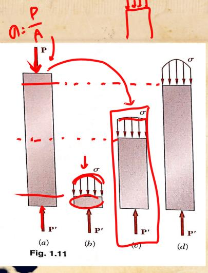
• In a slender rod subjected to equal and opposite concentrated load P ad P' (Fig.1.11*a*), this variation is small in a section away from the points of application of the concentrated loads (Fig. 1.11c), but it is quite noticeable in the neighborhood of these points (Fig 1 11h and d)
