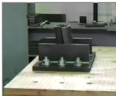
図-6 変形後の鞘管
